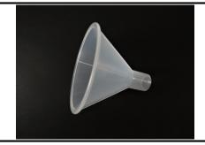
**1. General description:** Made of PP, with ribbed outside to avoid pressure build-up. Angle of inclination 60°. Autoclavable.
