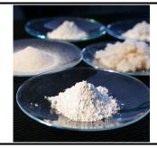
**1. General description:** DMT beech wood dust is used to measure vacuum, cleaning interval and
