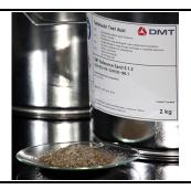
**1. General description:** The DMT CN / ISO reference sand is specified in both ISO 679 and DIN EN 196.
