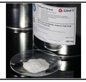
1. General description: For the testing of gas turbine and diesel engine filters, these are often tested according to Aramco standard 32-SAMSS-008. The Aramco test dust specified in the above standard is used for this purpose. The specification specifies that the particle size distribution of sodium chloride in the test dust must be between 0-5 µm. The DMT GmbH & Co. KG produces DMT Aramco test dust using a special process so that the sodium chloride, which can become highly agglomerated at
