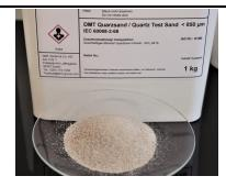
1. **General description:** Standard 60068-2-68 defines test procedures to determine the effects of dust and sand as an air component on electro technical products. DMT quartz sand < 850 µm is used for the Lc test according to methods Lc1 and Lc2.
