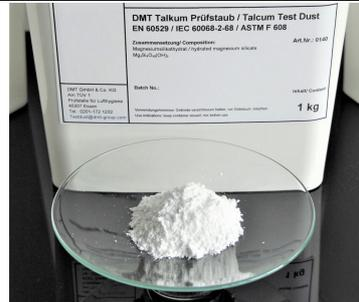
**1. General description:** DIN EN 60529 provides a system for classifying the degrees of protection of electrical equipment. DMT talcum test dust is used for the dust test for the first code numbers 5 and 6 in accordance with Chapter 13.4.
