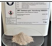
**1. General description:** DMT dust is the dry mixture according to 78/318/EEC used for the test liquid.
