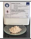
**1. General description:** DMT dust is the dry mixture according to 78/318/EEC used for the test liquid.
