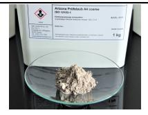
**1. General description:** The coarsest test dust of ISO 12103-1 is the Arizona test dust A4 coarse.
