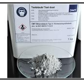
**1. General description:** DMT mineral dust type 4 is used for testing according to chapter 5.11.
